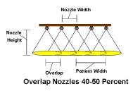
Figure 2. Nozzle overlap for flat fans.
