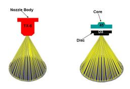
**Figure 4.** Hollow cone nozzles — nozzle body and disc-n-core
