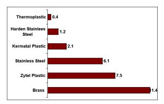
Figure 5. Percent increase to nozzle flow rate of flat fan spray.
