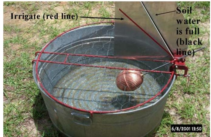
Figure 6. Operating positions for the unit.
