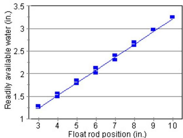
Figure 5. Relationship between the position on the float rod and the depth of water to be removed before irrigating.
