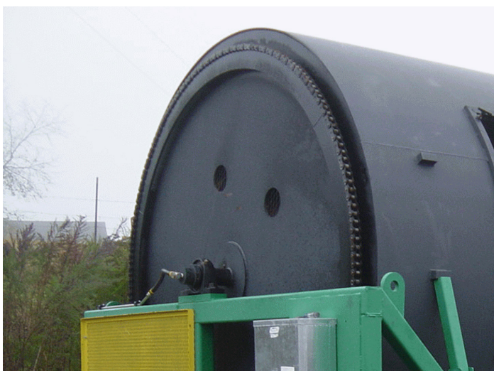
Figure 5. In-vessel rotary composter with forced air infusion capabilities. [Courtesy Industrial Piping, Inc.]
