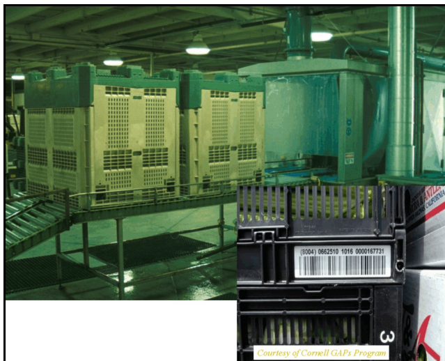
Figure 41. Barcoding facilitates trace-back and sanitizing of RPCs.
