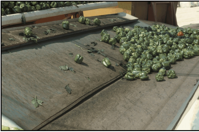
Figure 36. Padding along the conveyor minimizes damage to peppers when they are dumped from bins.
