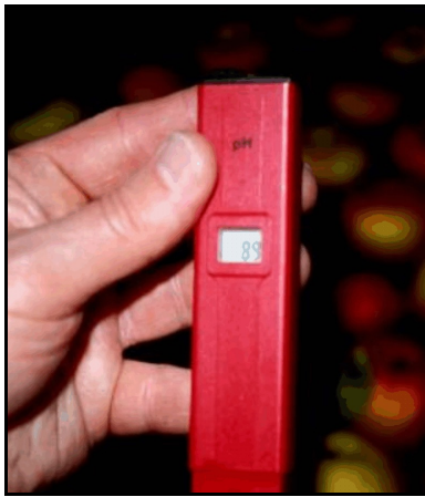
Figure 40. Testing pH regularly will help maintain the maximum disinfectant activity of chlorine in wash or cooling water.
