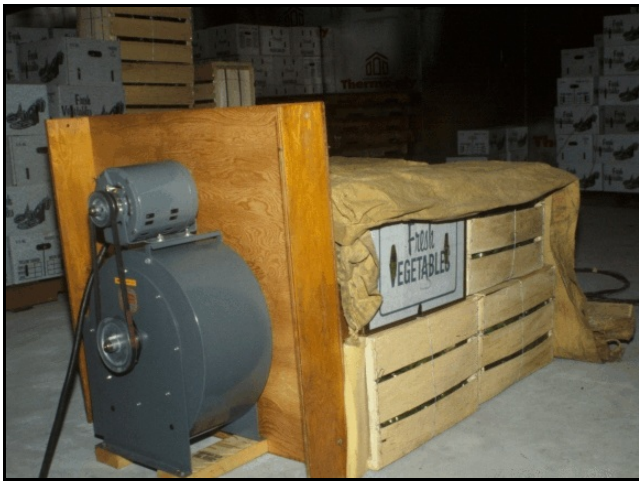
Figure 42. An effective portable forced-air cooler for small operations can be constructed with plywood, a tarp and a squirrel-cage fan.
