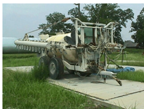
Figure 1. Air-assisted boom sprayer.
