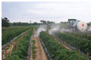
Figure 2. Hydraulic boom sprayer.
