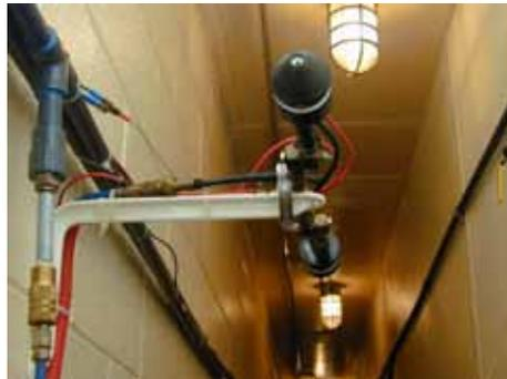
**Figure 2.** Electrostatic spray nozzle in a hatchery plenum.
