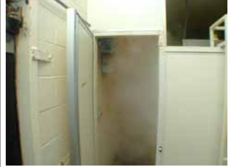
**Figure 4.** Electrostatic application of sanitizer in a hatchery plenum.
