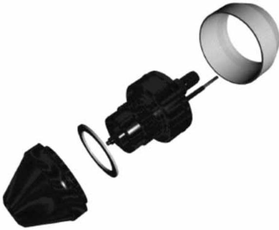
**Figure 1.** Electrostatic Spray Nozzle.
