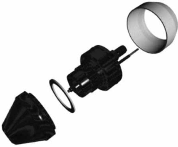
**Figure 1.** Electrostatic Spray Nozzle.
