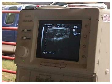
**Image 2:** The ultrasound machine displays the reflected sound waves as an image on the screen. This is a ribeye image.
