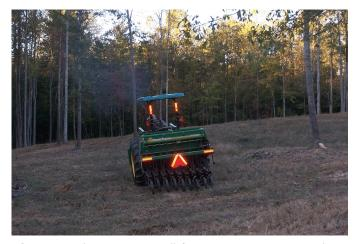
**Figure 5.** Planting a NE tall fescue into a suppressed sod with a no-till drill. Photo Credit: Di Hodges.
