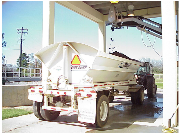
Loading and transporting biosolids from a wastewater treatment plant to the farm.
