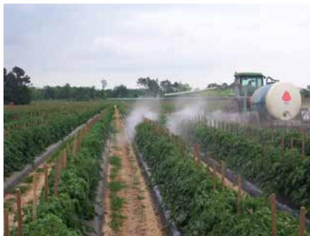
Figure 2. Hydraulic boom sprayer. The sprayer shown here is applying pesticides to tomatoes, but the spray is the same for snap beans.
