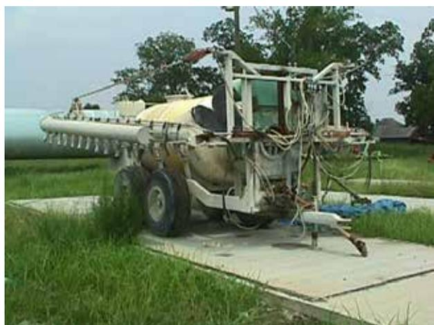
Figure 1. Air-assisted sprayer for insect and fungicide application.
