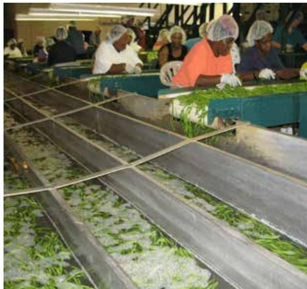
**Figure 3.** After field trash is removed, beans are graded, then cooled in water flume.
