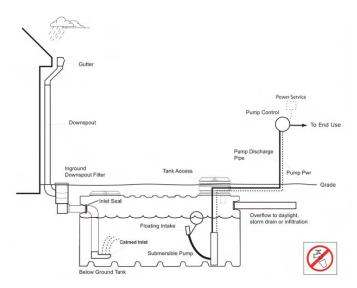
Fig. 3: Below ground system (Van Giesen and Carpenter 2009)
