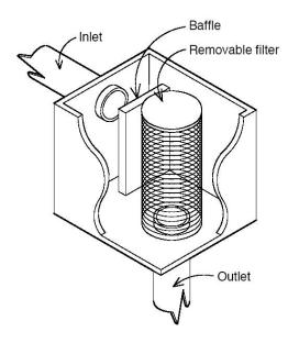
Fig. 4: Box filter (Texas Water Development Board 2005)
