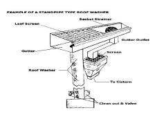
Fig. 5: Roof washer (Van Giesen and Carpenter 2009)
