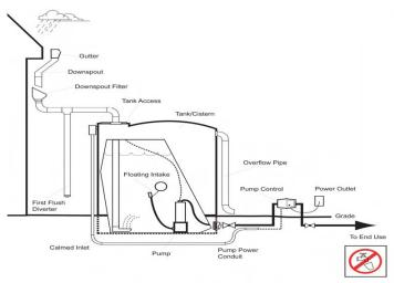
Fig. 2: Above ground system (Van Giesen and Carpenter 2009)
