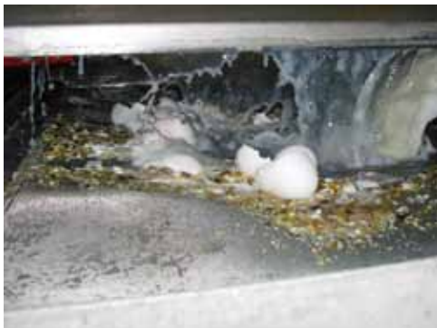
Figure 7. A manual static screen is used just below an egg washer to capture grit particles early in the shell egg cleaning, grading and packaging process. This early intervention step will significantly reduce the amount of grit entering the wastewater treatment system.
