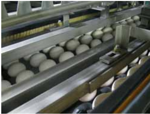
Figure 6. Taking the time to observe egg washers during operation can help processors identify needed adjustments if excessive breakage is occurring during the washing process.
