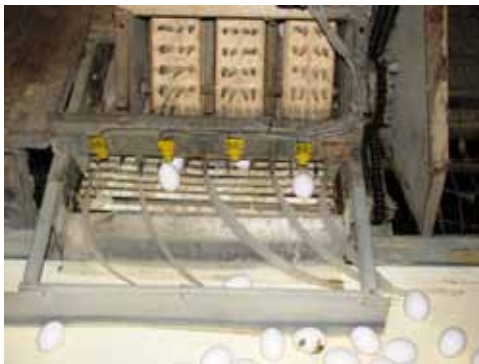
Figure 4. Minimizing egg breakage begins in the layer house. Here, flexible plastic strips are used to ensure a smooth transmission of eggs onto the processing plant transfer belt. Without the aid of the plastic strips, eggs would roll unchecked onto the belt, increasing breakage.
