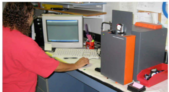
Figure 5. Analyses that once took numerous hours in the laboratory can now be performed in seconds using near infrared (NIR) spectroscopy. Though wet chemistry methods are still performed to check the calibration of the NIR system, the main forage quality measurements can now be accurately made at relatively low cost.
