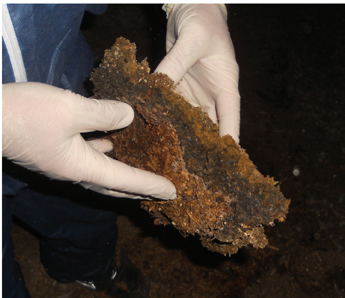
Figures 5 and 6. Caking of pine shaving (Figure 5) and caking of GMG (Figure 6).
