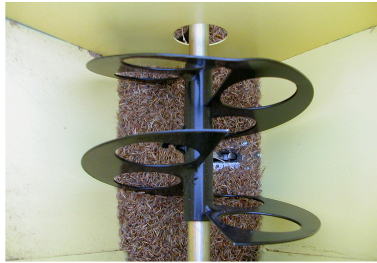
Figure 2. Agitators in the bottom of native grass hopper boxes ensure that the fluffy appendages on the seed of some native prairie grasses do not keep the boxes from properly metering the correct rate.
