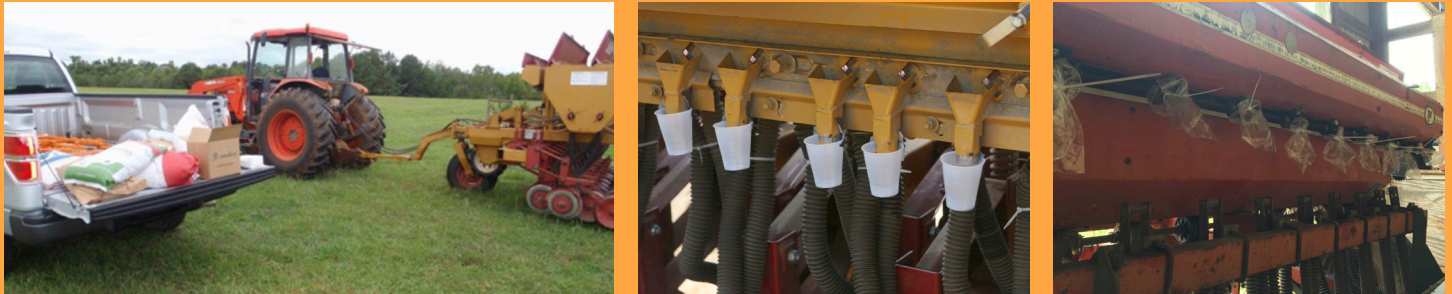
Figure 9. Before beginning, assemble all the supplies that one will need. Plastic storage bags or cups can be used to catch the seed. If secured to the metering units with duct tape or cable ties, care must be taken to ensure that the drop tubes are free of obstructions by dropping a few seeds down the drop tubes to ensure that they drop through easily.
