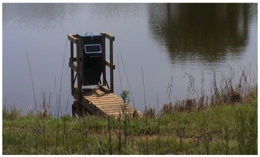
Figure 8. A fish feeder, placed on a dock for easy access, is activated by a timer and solar powered.
