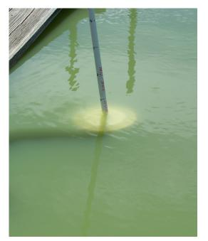
**Figure 6.** Using a white target on a stick to measure light penetration into pond water. The best range of light penetration is between 12 and 18 inches when using a pond fertilization program.
