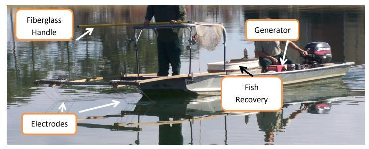
Figure 12. Electro-fishing equipment used to check pond balance or relocate fish.
