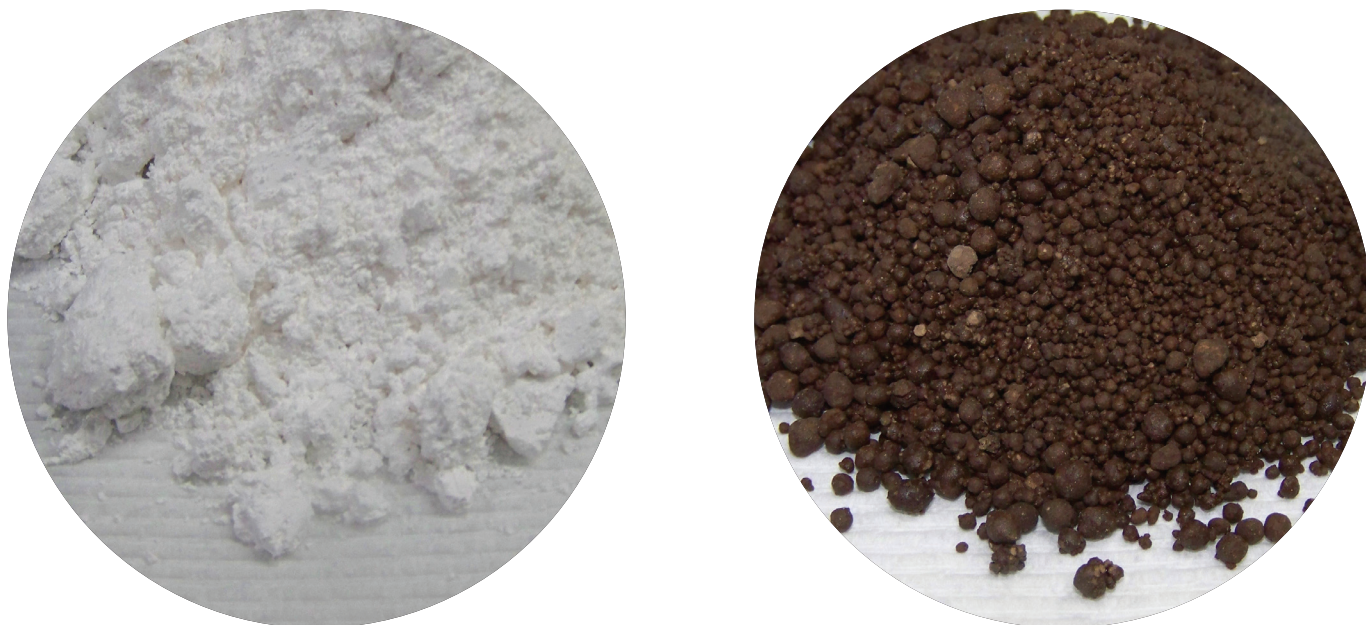
Figure 2. Finely powdered lime (left) and pelletized lime (right) dissolve over several months in pond water.
