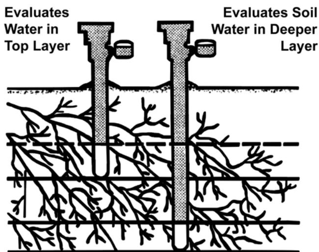
Figure 2. Typical Tensiometer Location
