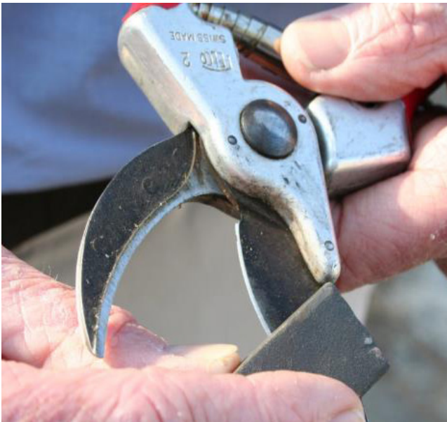
Figure 8. Proper sharpening of bypass hand clippers.
