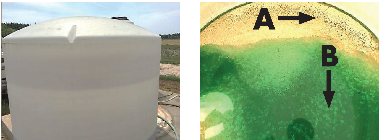
Figure 7. Fertilizer feed tank that has not been cleaned or winterized, from the outside (left) and inside (right). See fertilizer salt deposits (a) and evaporated and precipitating fertilizer (b).
