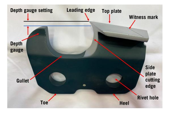
A diagram of the parts of a chainsaw cutter is below.
