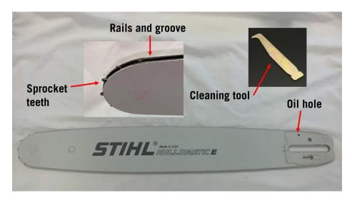
length down on a flat surface and look for light underneath it. If the bar is curved, it is time to replace it.
