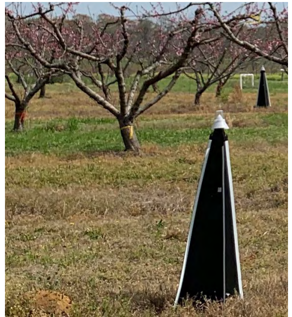
Figure 4. A modified Tedder's trap, also known as a black pyramid trap, used for monitoring adult plum curculio activity in orchards.
