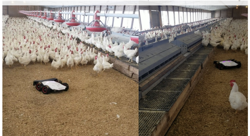
Figure 5. Robotic application for reducing floor eggs in broiler breeder houses from an ongoing study by UGA poultry science researchers.
