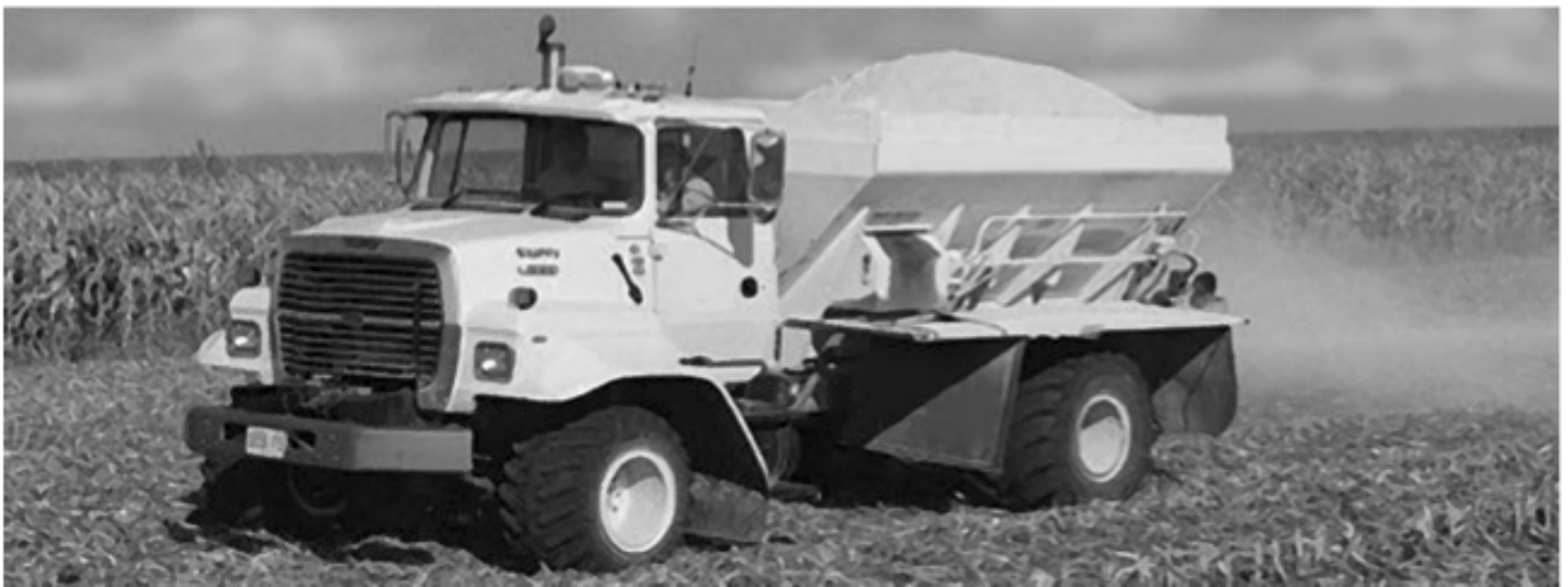
Lime applied by a truck.
