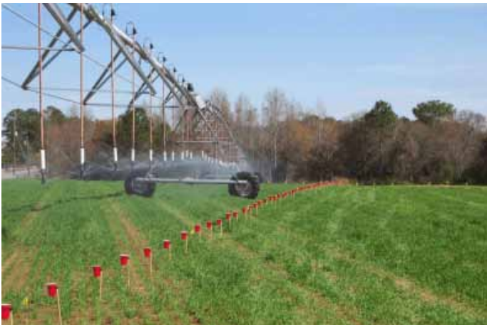
Figure 1. Catch cup layout using 16-ounce drink cups as collection devices.
